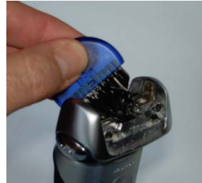
Figure 6: Cleaning the Shaving Head Base
