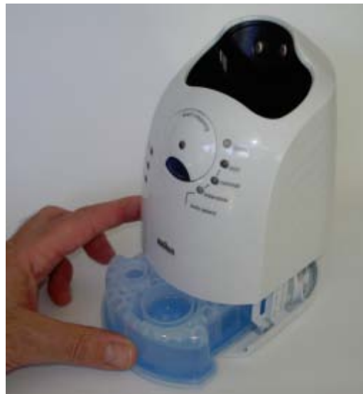
Figure 18: Sliding in New Cartridge
