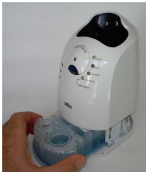
Figure 16: Sliding Out Old Cartridge
